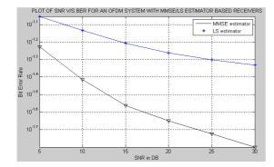
Figure 5: BER v/s SNR for SISO OFDM System
