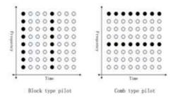
Figure 3: Block and Comb Type Pilot
