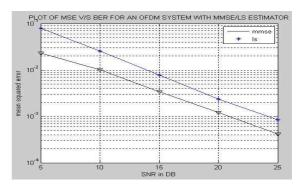
Figure 6: MSE versus SNR for SISO OFDM System
