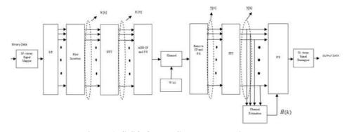
Figure 1: SISO OFDM System Block Diagram
