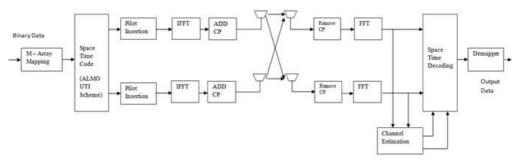
Figure 2: MIMO OFDM System Block Diagram
