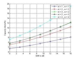
Figure 4: Channel Capacity v/s SNR for SISO and MIMO OFDM System
